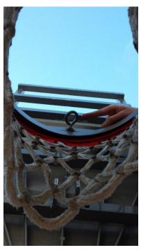
5. Connect the connector pole to the **bottom** bracket of the modified hoop and tighten the I bolt
